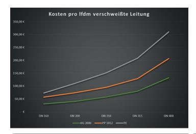
Sample cost comparison: Pipes according to DIN EN 1852 and DIN EN 14758 (KG 2000) welded with IP-plus welding system, compared to welded PE-HD wastewater pipes of the same ring stiffness. This shows the significant cost savings of 25-40% in the total cost consideration. (depending on diameter)
