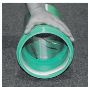
The IP-plus welding ring is so simply designed that it can be installed professionally in just a few steps. The existing rubber sealing ring is replaced by the IP-plus welding ring and then welded with an electric welder.
